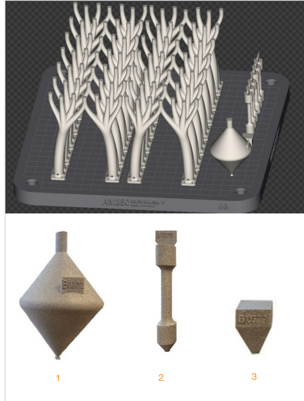
Figure 3. An example of a build setup with 1. powder capture capsule, 2. tensile bars (x6) and 3. density block
