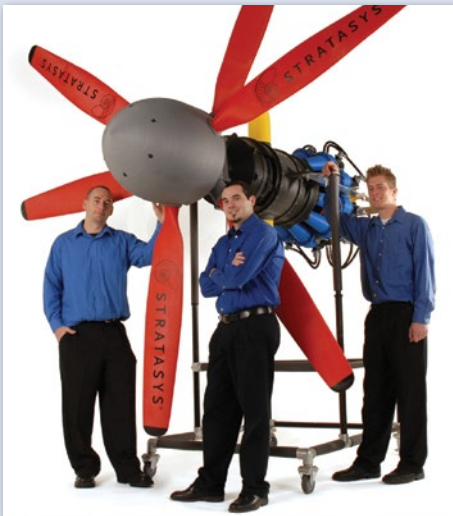
In 2009, Stratasys (Minneapolis & Rehovot, Israel) and Autodesk (San Rafael, CA) unveiled the first full-scale turbo-prop aircraft engine model produced using Stratasys FDM (Fused Deposition Modeling) technology, a form of AM.
